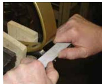
2. To fix profile, file over and down. For width and thickness, file flat on the underside only. Do not file the radius to sharpen.
