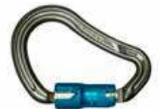
Aluminum Carabiner 5555S2 Length: 4.80" (122mm), Opening: .78" (20mm), Breaking Strength: 6,744 lbs. (30kN)
