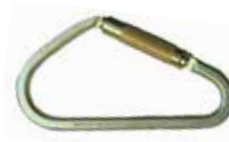
Steel Carabiner 5005L1 Length: 7 5/8" (193.68mm), Opening: 2 1/8" (53.98mm), Breaking Strength: 8,992 lbs. (40kN)
