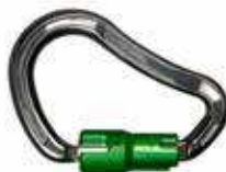
Aluminum Carabiner 5555S3 Length: 4 7/8" (123.83mm), Opening: 3/4" (19.05mm), Breaking Strength: 6,744 lbs. (30kN)
