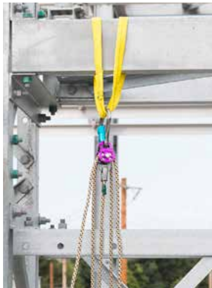
2. Raise victim with Rescue Blocks and progress capture.
