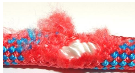
Excessive Abrasion / Wear Contrasting Core visible
