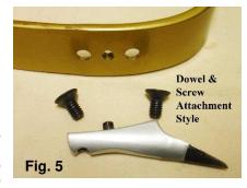
first time removed, but if re-using, apply a low to medium strength thread sealant (Loctite® or equivalent) to prevent the screws from loosening. Screws may not be removable if a permanent type thread sealant is used.
