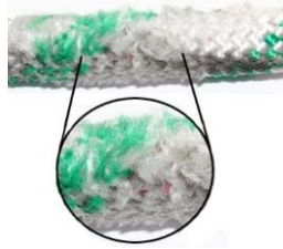
Rope with Excessive Abrasion Wear
