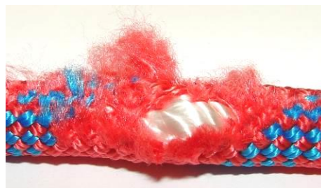
Excessive Abrasion / Wear - Contrasting Core visible
