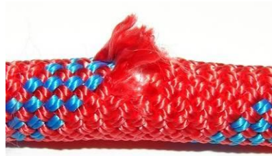
Broken or Cut Strands
