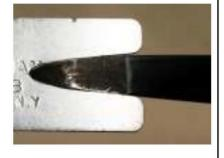
Do not use as a precise measurement but as a guide to prevent shaping the gaff too narrow. When gaff tip is inserted in gauge as shown, the gaff should not pull through the slot. If gaff pulls through the slot the gaff has been shaped to narrow to be used safely.
