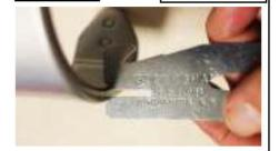
If at any point along either edge, the stirrup portion of the climber fits into the Stirrup Thickness Slot, the climber is too worn to be used safely.
