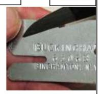
Slot should be your GUIDE to proper shaping of the gaff tip. A reasonable snug fit with the tip radius closely matching that of the slot may be considered proper. A gaff tip that fits loosely and ends in a sharp point without the radius is unsafe for climbing. Such a gaff should be re-shaped gradually, as shown in the Reshaping Instruction section.
