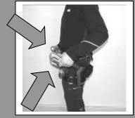
For part time attachment of the Batten Seat to the Ergovation<sup>®</sup> saddle / sit harness: This requires 2 ANSI, OSHA, CE, etc. compliant carabiners (pictured left) for suspension support connection to your saddle / sit harness.
