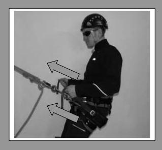
To raise or lower the Batten Seat, adjust each side strap of Batten Seat until it is snug against buttocks of user.
