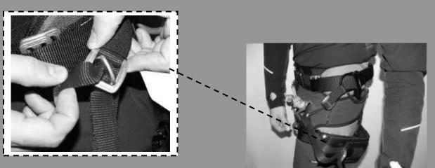
To attach buckle and strap from Step 4B to mating attachment of Batten Seat, turn buckle at an angle and push from the bottom out through larger buckle frame as pictured above. Repeat Step 4B & 5B for attachment of the opposite side of Batten Seat.
