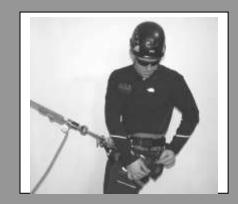
Once the batten seat is properly adjusted tuck excess webbing to prevent from catching in climbing system.
