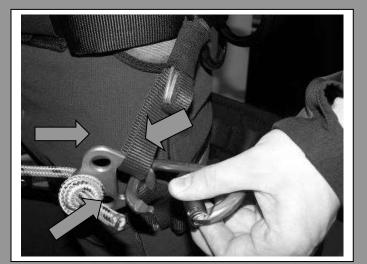
Attach carabiner of one end of Batten Seat to any load bearing connection of the Ergovation<sup>®</sup> saddle / sit harness's approved suspension points. Attach the second carabiner of the Batten Seat to an equivalent load bearing connection of the Ergovation<sup>®</sup> saddle / sit harness's opposite side.
