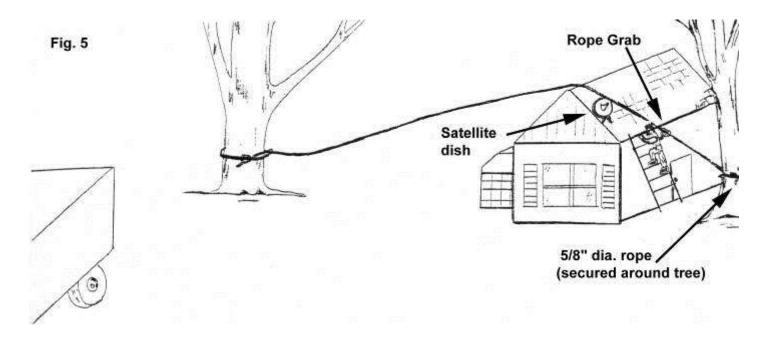
10. To aid in allowing the rope grab to easily slide down the rope as you come down the roof and ladder, you can hold the trip lever cam on the rope grab open. If you slip, remove your hand and the ascender rope grab will lock, stopping your fall.
