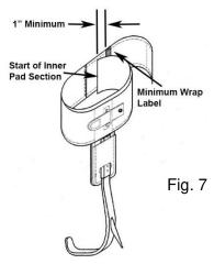
Note: Do not use product if the minimum wrap label cannot be pulled at least 1" past the start of the inner pad section. Contact Buckingham Mfg. for alternate option.
