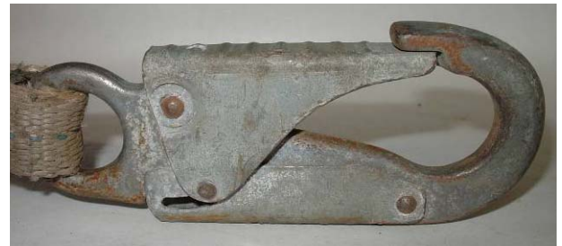
EXCESSIVE WEAR OF HARDWARE OR CRACK (Cracks are indicated by fine black lines)
