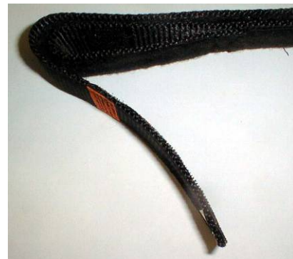
HOOK AND LOOP DOES NOT ADHERE
