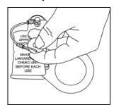
1. Depress the button on the safety locking pin and remove from main assembly.
