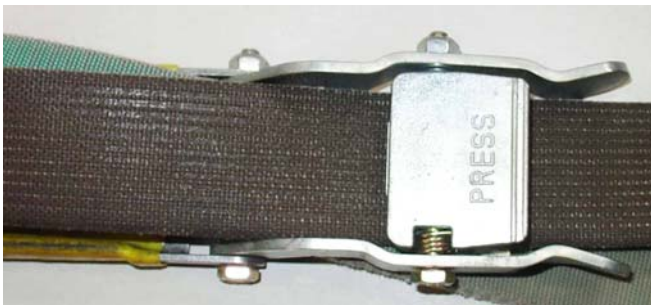
Nuts Are Properly Attached and Securely in Place
