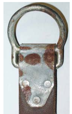
Broken / Missing Rivet
