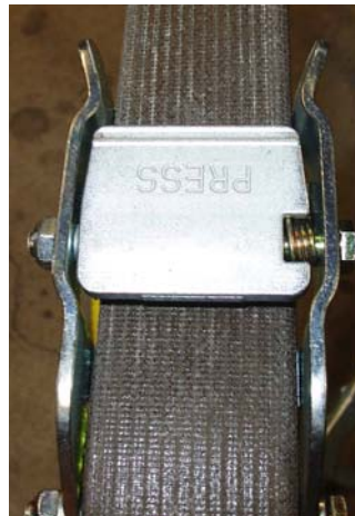
Cam Buckle Properly Locks and Is Free of Foreign Objects
