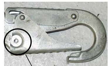
Broken / Missing Rivet
