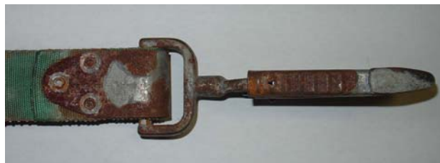
Rusted / Excessively Corroded Hardware
