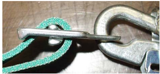
Friction Buckle Properly Locks and No Slipping of Inner Strap.
