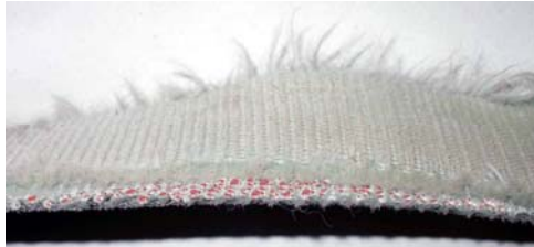
Red Warning Center Exposed (Woven Inner Strap)
