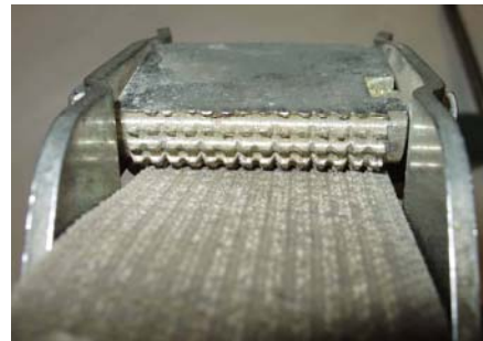
Cam Buckle Properly Locks and Is Free of Foreign Objects
