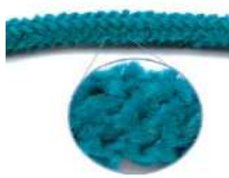
Rope with Excessive Abrasion Wear
