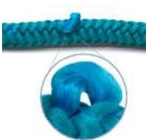
Rope with a Pulled Strand
