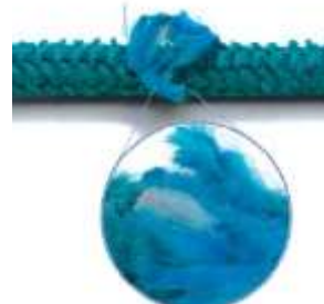
Rope with Broken or Cut Strands
