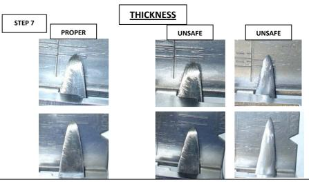
If the gaff tip, when inserted through each of the Thickness Check Steps, fails to fit between the inscribed lines on the gauge, the gaff is either:
