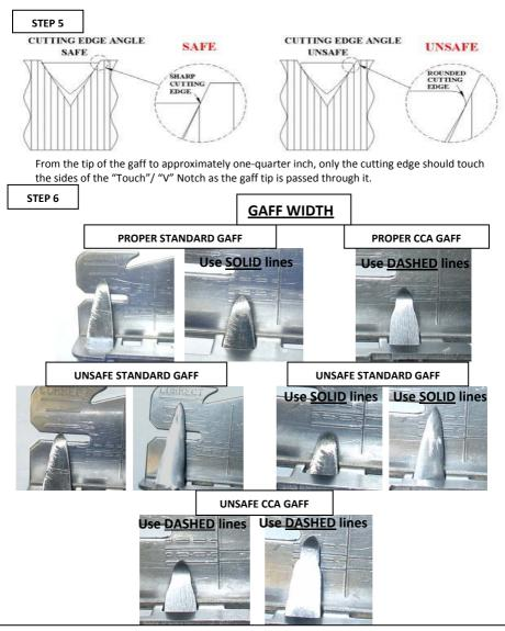
**Note**: When checking a <u>CCA pole gaff</u> for the 1/2" width dimension, (smaller of two width windows) the gaff tip should fit between the dashed inscribed guide lines on the gauge. All other windows/steps are to be used for both CCA & Standard pole gaff inspections.
